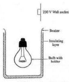
Figure shows some of the apparatus provided to you to experimentally determine the electric power dissipated as heat from a 230 V, 25 W filament bulb. You are asked to use water to collect heat given out by the bulb.
